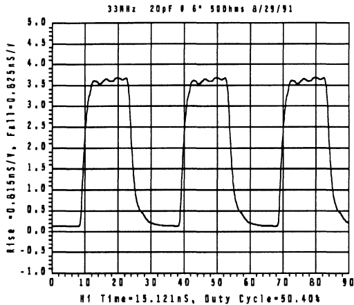
20 pF Load with 6" of Trace ( Z_0=50\Omega ) Single Driver
